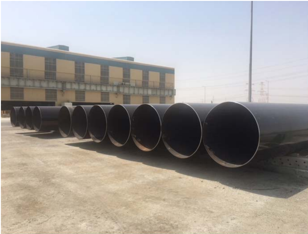
Large diameter, welded steel pipe manufactured by AGPC
